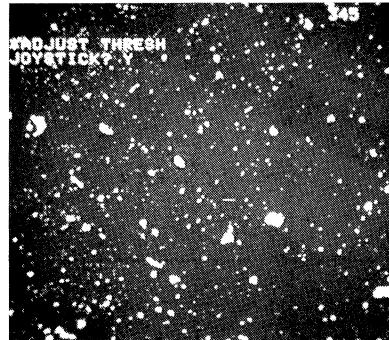
After calibration, objects in the field are uniformly extracted, but noise is still apparent. This noise tends to mask the presence of small objects.
